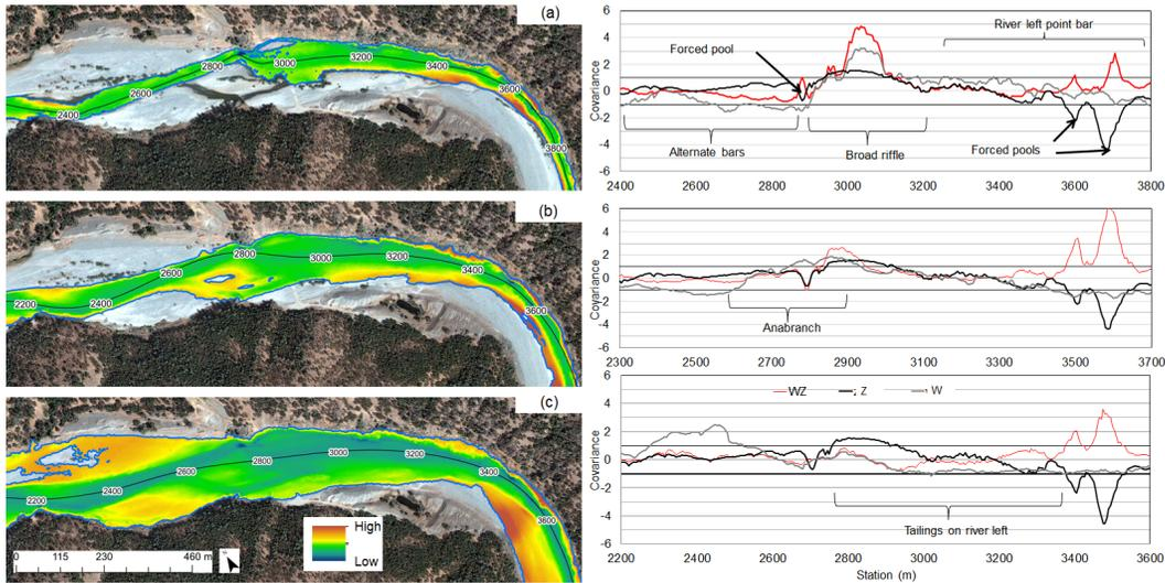
**Figure 5.** Example section of detrended bed topography and plots of  $Z$ ,  $W$ , and  $C(Z, W^j)$  for  $8.50 \text{ m}^3 \text{ s}^{-1}$  (a),  $283.2 \text{ m}^3 \text{ s}^{-1}$  (b),  $3126 \text{ m}^3 \text{ s}^{-1}$  (c) at the lower extent of the study area. The detrended topography has been clipped to the wetted extents for each flow to accentuate relative bed features. Flow dependent sample pathways are shown for stationing reference between the image and the plots.
