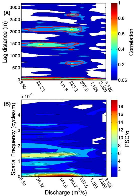
**Figure 9.** Autocorrelation **(a)** and PSD **(b)** of  $C(Z, W^j)$  with increasing flow. For the ACF plot **(a)**, only values exceeding white noise at the 95 % level are shown and the red contour demarcates the 95 % level for an AR1 process (red noise). For the PSD plot **(b)** only values exceeding white noise at the 95 % level are shown.
