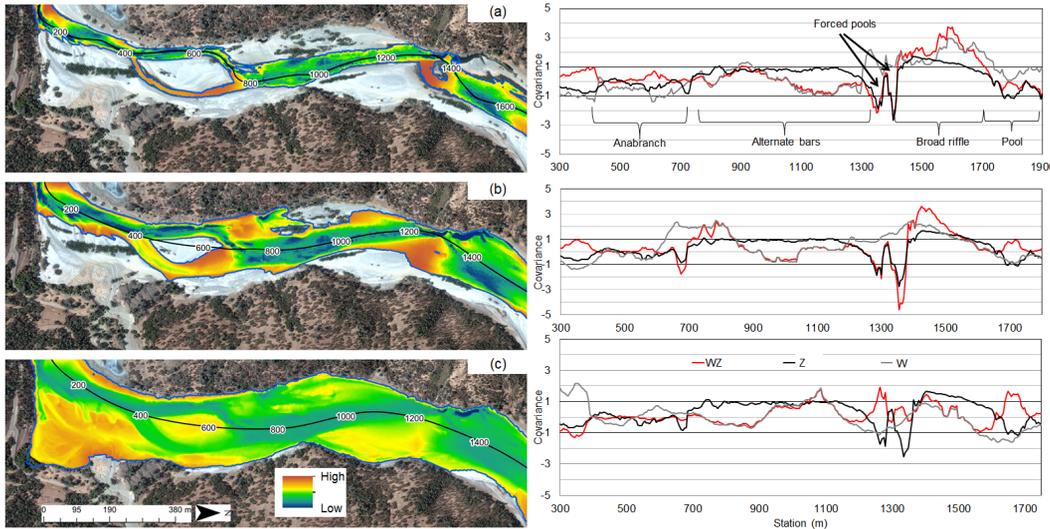
**Figure 4.** Example section of detrended bed topography and plots of  $Z$ ,  $W$ , and  $C(Z, W^j)$  for  $8.50 \text{ m}^3 \text{ s}^{-1}$  (a),  $283.2 \text{ m}^3 \text{ s}^{-1}$  (b),  $3126 \text{ m}^3 \text{ s}^{-1}$  (c) in the middle of the study area. The detrended topography has been clipped to the wetted extents for each flow to accentuate relative bed features. Flow dependent sample pathways are shown for stationing reference between the image and the plots.
