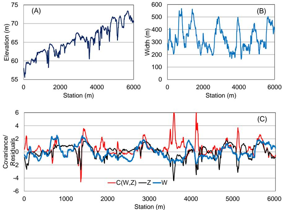
**Figure 2.** Raw bed profile **(a)** and flow width **(b)** series for  $283.2 \text{ m}^3 \text{ s}^{-1}$ . After detrending and standardizing both series values of  $Z$  (black line in **c**) and  $W$  (blue line in **c**) are multiplied by each other generating the  $C(Z, W^j)$  GCS (red line in **c**).
