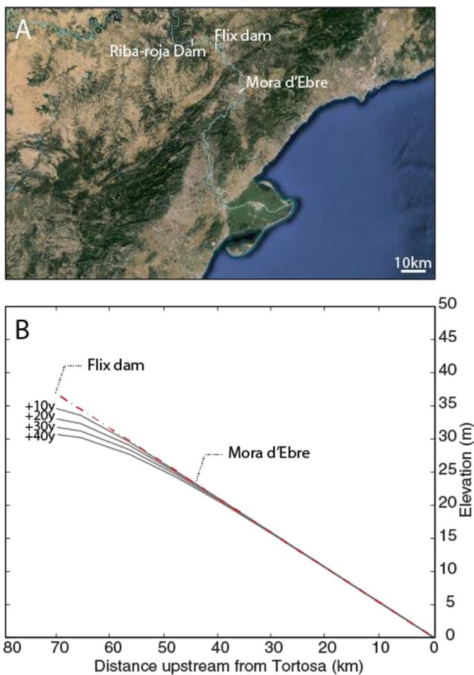
Figure 6. (A) A close-up of the Ebro drainage basin close to the delta (data from Google Earth, 2015). (B) Modeled response of the Ebro River downstream of the lowermost modern dam, the Flix dam. The bed degradation measurements from Vericat and Batalla (2006), are taken 25 km downstream of the Flix Dam, in Mora d'Ebre.
