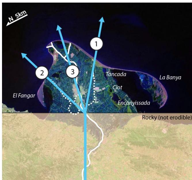
5 **Figure 2.** Schematic of modeling scenario, highlighting the succession and orientation of Ebro delta lobes, shown on top of the modern Ebro delta morphology (NASA Landsat image) and the inferred paleo channels (dotted lines, from Maldonado, 1975). In the model, the straight reference coastline is assumed to be non-erodible. Names refer to the spits and the lagoons on the Ebro delta. Numbers refer to the (1) Riet Vell, (2) Sol de Riu, and the (3) Mitjorn-Buda lobes.
