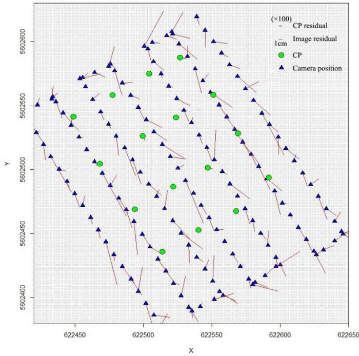
Figure. Residuals on the images and CPs in planimetric view (vectors give the horizontal residual component magnified by  $\times 500$  and  $\times 100$  for DSLR and action camera, respectively).
