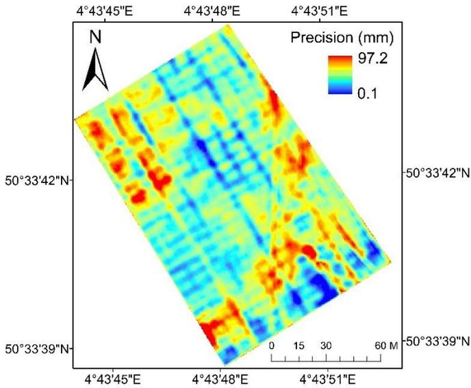
*Figure. Precision map estimated based on Monte Carlo and tie point density. The XYZ error was estimated by the density-error regression model ( $y = -0.00041x + 0.125$ )*
