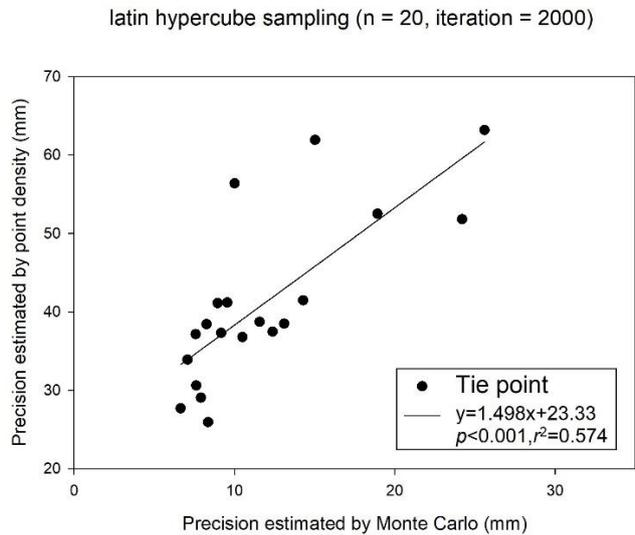
5 Therefore, the estimation based on tie point density could be a quick alternative approach of evaluating tie point precision and spatializing the error.
