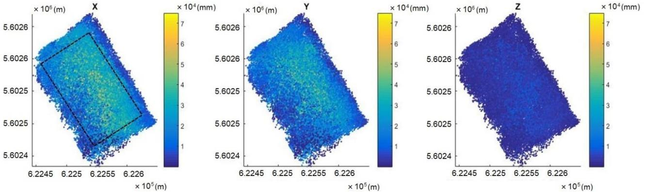
Figure. Precision and error maps for simulated UAV surveys. The region encompassed by the dashed line is the same processing area of the propagated error maps based on tie point density.
